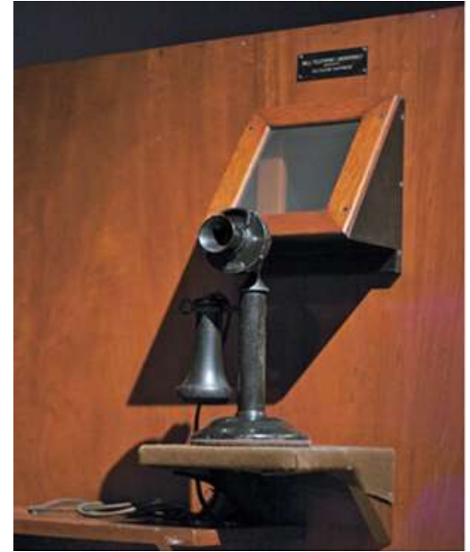
Bell Labs video phone prototype (1927)
