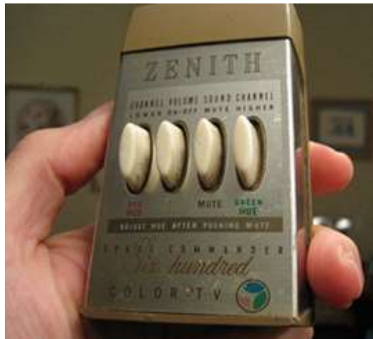
Zenith Space Commander 600 wireless TV remote control (1956)
